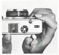
Advance film and release shutter until No. 1 appears in exposure counter window.
