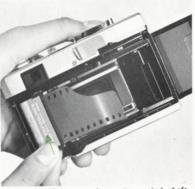
Insert film magazine onto rewind shaft,
