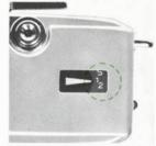
The film counter shows S, 1, 2, 4 and subsequent even numbers up to 36. The numbers 12, 20 and 36 are in yellow color. Each time the film is advanced, the counter counts up the number of exposures made, which is marked by the orange color arrow ( ). When the rear cover is opened, the counter returns automatically to S.
