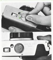
For correct camera operation, the mercury battery must be properly inserted into the battery compartment at the bottom of the camera.
