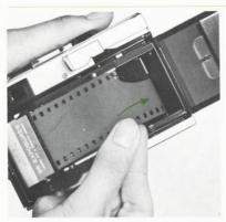
Insert film leader into one of the slits on easy load take-up spindle.
