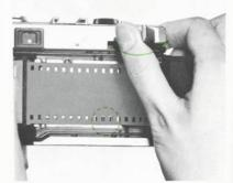
Advance film until it is securely placed between film guide pins. Make certain sprocket wheel engages in perforation in film properly before closing rear cover.
