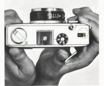
Advance film by rotating film advance lever and depressing shutter release button alternately until No. 1 appears in film exposure counter window on top of camera.
