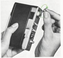
After the entire roll of film is completely exposed, depress the rewind button, rewind film into magazine and remove. (See page 28.)
