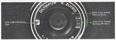
Depress ASA ring in the front of camera slightly and rotate it around the lens to select ASA (or DIN) rating for your film. For perfect exposures, the correct ASA or DIN film speed of your film must appear in the ASA setting window. The window is in the right side of the lens as viewed from the front.
