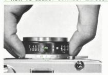
The characteristics of 35RC will be fully appreciated in auto-exposure photography. When you set the F/stop ring to the mark A, a proper lens aperture is automatically combined with your predetermined shutter speed for correct exposure. In automatic exposure the shutter speed must be predetermined, depending on shooting conditions, and this shutter speed will automatically control the F/stop for proper exposure. (See page 17.)
