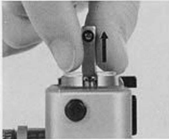
2. Place film cartridge into the film cartridge chamber. If film rewind key does not engage properly in end of cartridge, rotate film crank in either direction until it does so.
